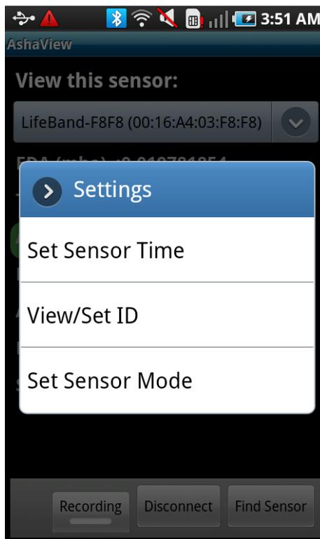
Next select “View/Set ID.” Press the field under the instructions to display the keypad and enter the new Device ID. The ID must be exactly 8 hex bytes (16 characters). 0-9 and A-F are permitted. When you have finished entering the new ID, press the Android Back button, then select “Update.” Ashaview will confirm that the device ID was successfully set.
