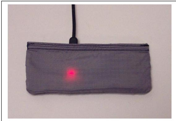
A standard micro-USB cable can be used to charge the battery. When the battery is charging, a steady red glowing light will be seen. The light will turn off (or grow very dim) once the charge is complete. The charging time may vary, but should be approximately 2-3 hours.
