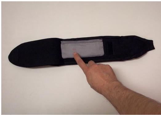
The LifeBand chest band is turned ON by pressing the tactile pushbutton located on the lower left side of the electronics pocket. (see photo)
