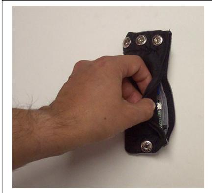
By pulling back the Velcro opening of the electronics pocket, the USB connector can be seen. (the small black device that can also be seen protruding from the electronics is the temperature sensor.)
