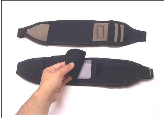
The Lifeband chest strap is a wearable wireless physiology measurement device. The Lifeband is designed for to transmit data to a mobile phone via the Bluetooth protocol.
